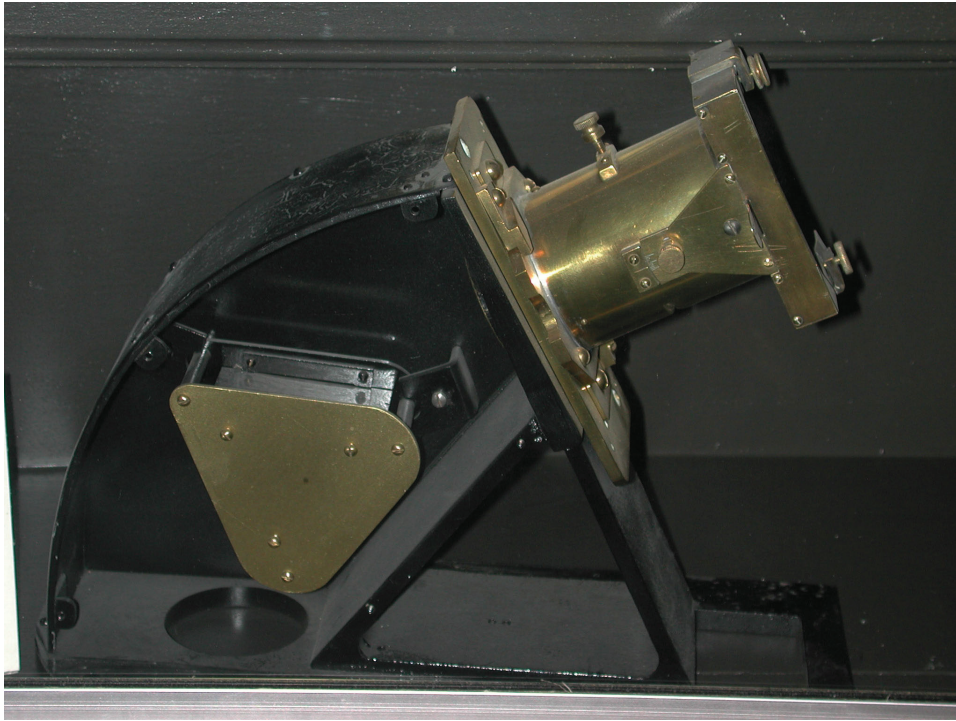
Figure 1. The collimated beam from the Brashear spectrograph enters from below through the hole on the lower left, passes through the prism (visible under the large triangular plate), and proceeds to the f/2.5 Voigtlander lens that is mounted inside the large brass cylinder in the upper right. The photographic plate holder is held under two mounting screws on the upper right hand side at the focal plane of the Voigtlander lens. The photo was taken by the author in the Lowell Observatory rotunda.
