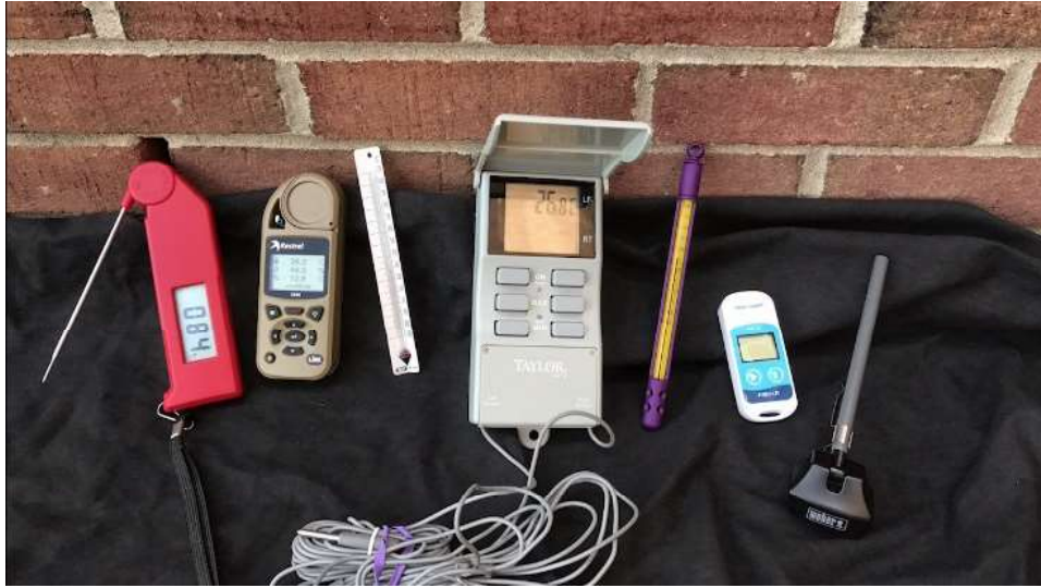
Figure 2. Sample thermometers tested by the GLOBE Observer team for use during the eclipse.
