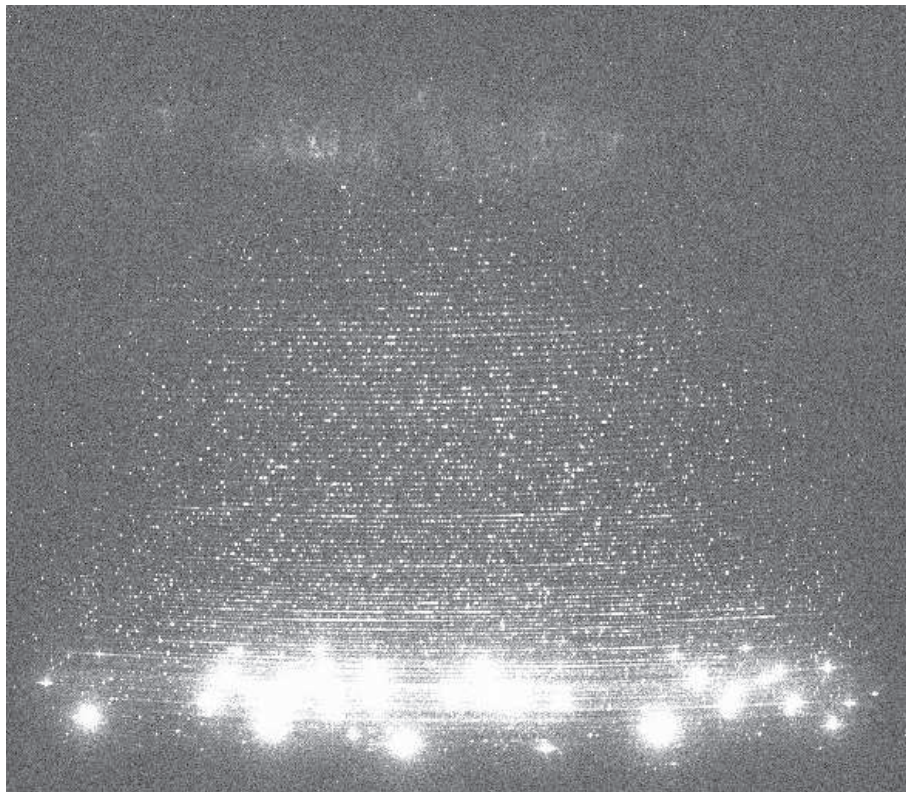
Figure 3. A spectrum of the Th-Ar lamp registered with the ARGES spectrograph (Wang et al. 2003).
