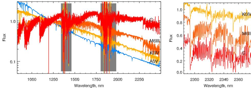
Figure 1. Data reduction quality provided by the FIRE pipeline. Left: Flux calibrated FIRE spectra of 4 stars having different effective temperatures and chemical compositions. Spectra are normalized to the flux at 1225 nm. Gray areas denote regions of strong telluric absorption. Right: Zoom-in on the NIR CO series for a K subgiant, late M giant, and a carbon star.
